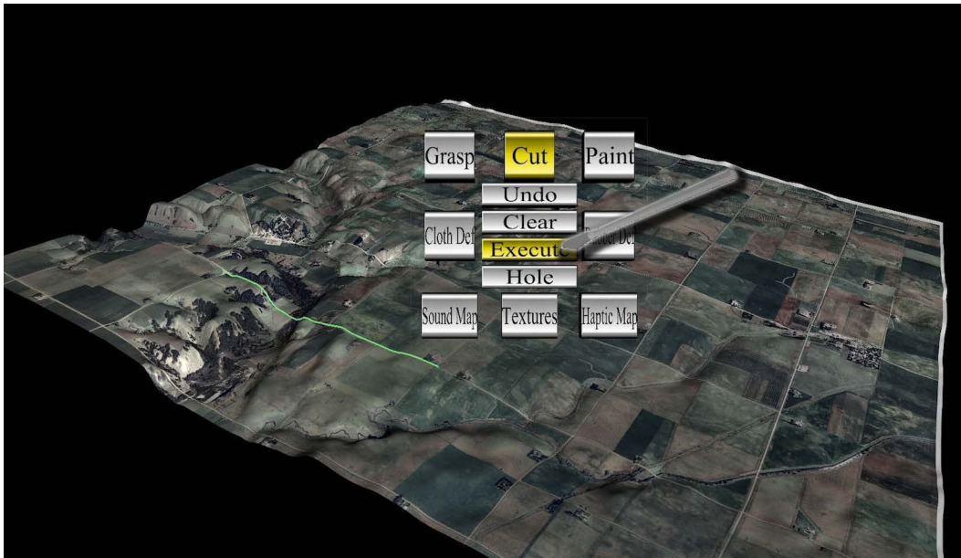
Figure 1.1 A stylus interacts with virtual buttons in a 3D interface
