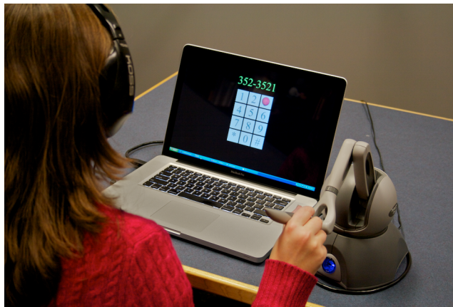
Figure 4.2 The experiment setup with PHANToM Omni.
